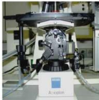
**Figure 2** Condenser for TIR illumination under variable angle; schematic (left) and laboratory equipment with an additional light path for transillumination and phase contrast microscopy (right).
