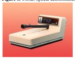
by means of optical densitometry. Optical density quantitatively describes the lightness or darkness of specific points on the X- film: one simply measures the transmission of light through a specific aperture on an optical densitometer (Figure 6). For example, if 1/5 of the light is transmitted (this area would appear quite transparent to light), then the optical density would be<sup>2</sup>
