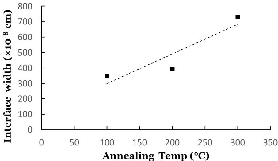
**Figure 4:** Interface width as a function of annealing temperature. The dashed line is the linear fit to the data. The interface increases linearly with temperature.
