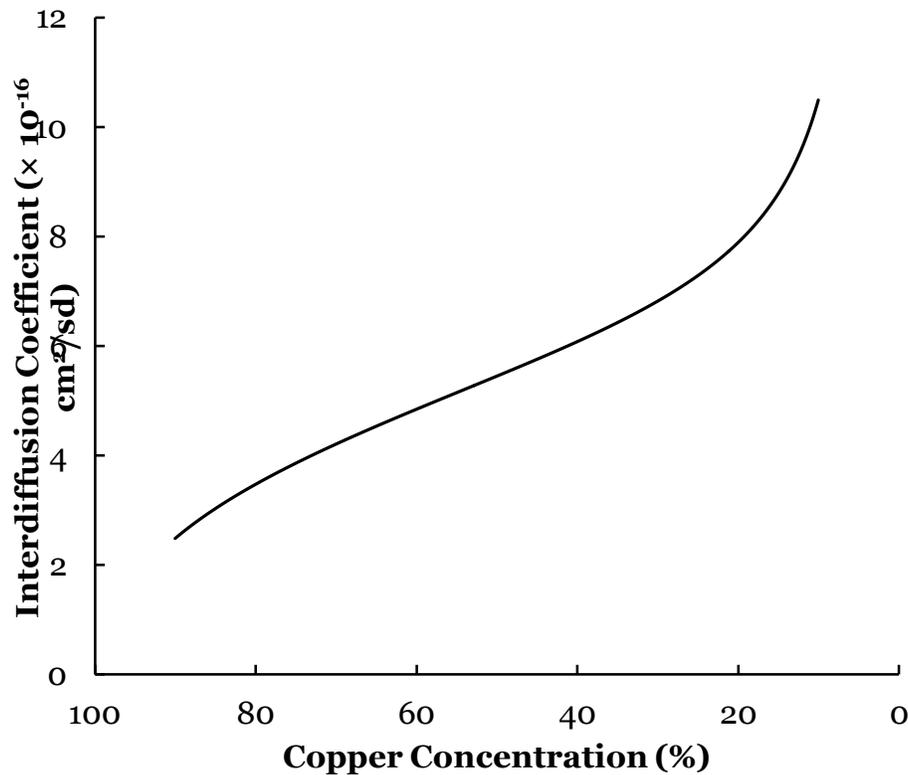
**Figure 6(a):** Interdiffusion coefficient as a function of atomic concentration of copper in the 100°C annealed sample calculated using equation (3).
