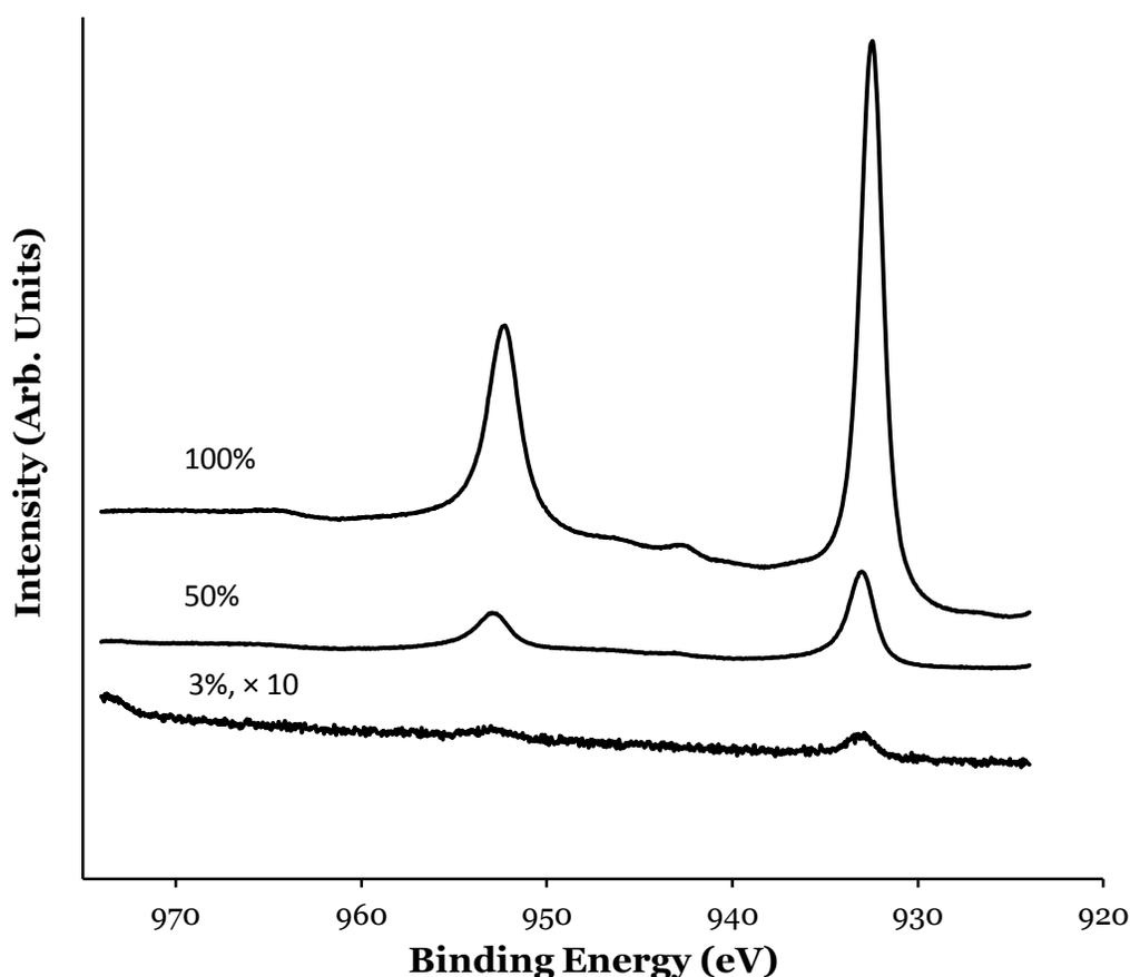
**Figure 1:** XPS spectra of copper 2p core levels in the 200°C annealed sample. The three spectra correspond to the regions in the sample where the atomic concentration of copper is 100%, 50%, and 3%.
