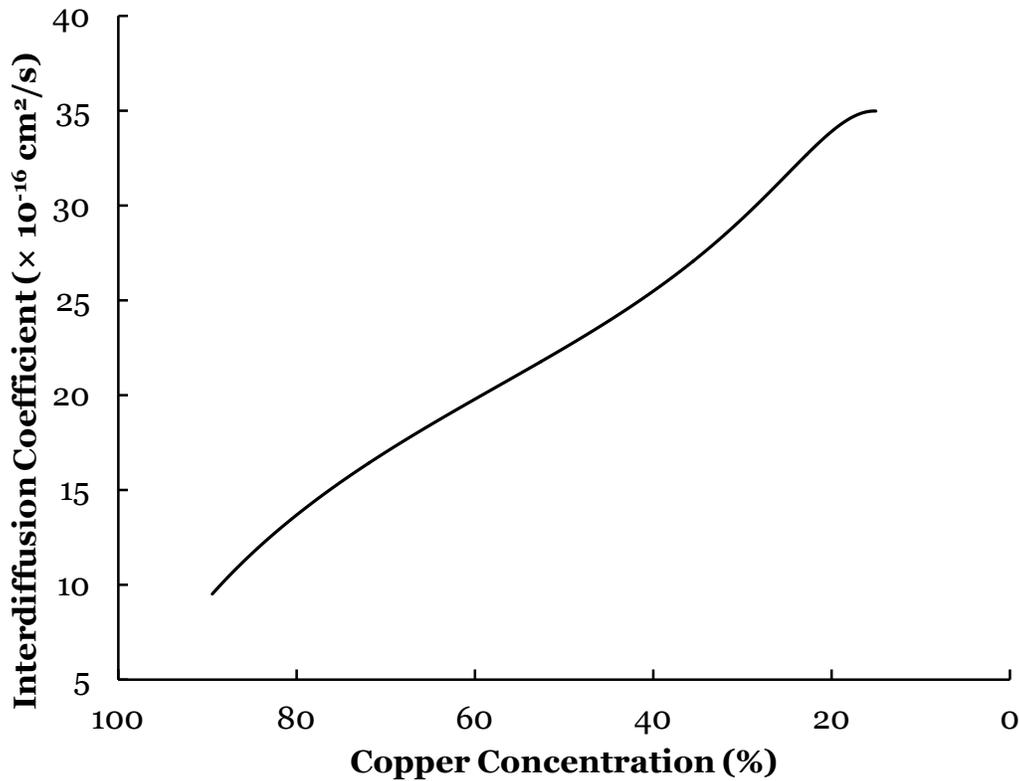
**Figure 6(c):** Interdiffusion coefficient as a function of atomic concentration of copper in the 300°C annealed sample calculated using equation (3).
