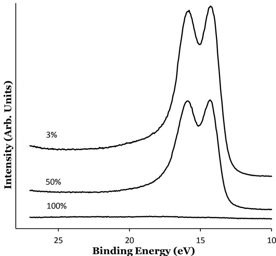
**Figure 2:** XPS spectra of hafnium 4f core levels in the 200°C annealed sample. The three spectra correspond to the regions in the sample where the atomic concentration of copper is 100%, 50%, and 3%.
