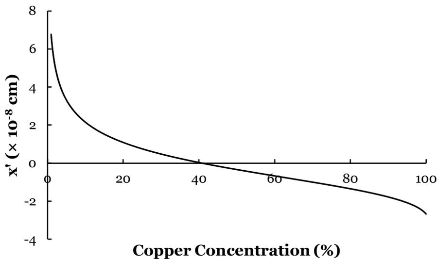
**Figure 5:** Percentage atomic concentration of copper as a function of depth referenced to the Matano plane, as determined using equation (2). The interdiffusion coefficient has been calculated from this figure.
