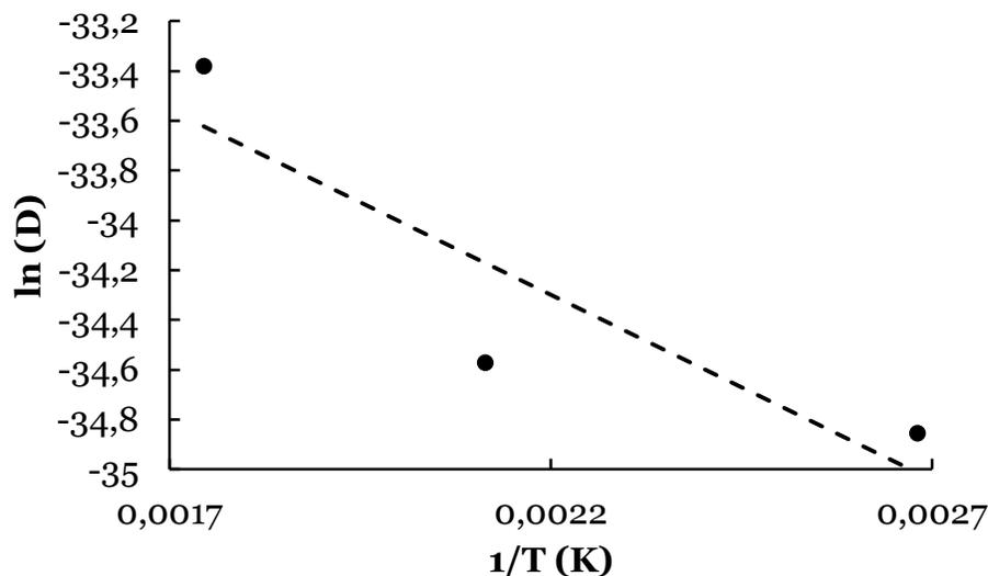
**Figure 7:** Arrhenius plot of the  $\ln(D)$  vs  $1/T$ . The dashed line is a linear fit to the data. The activation energy and the pre-exponential factor have been determined from the slope and the intercept of this line.
