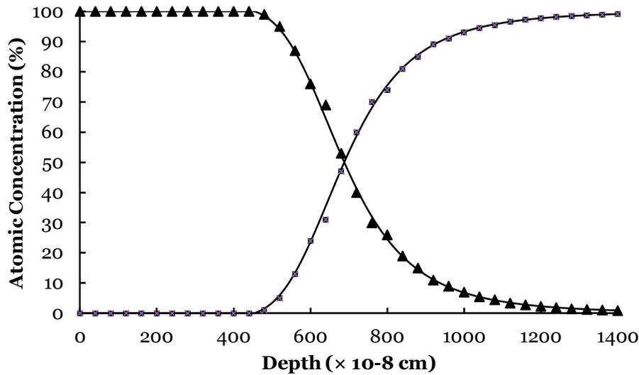
**Figure 3:** Percentage atomic concentration of copper and hafnium in the 200°C annealed sample as a function of depth. The markers represent the raw data. The triangles represent the copper and the squares represent the hafnium. The lines represent a fit to the raw data.
