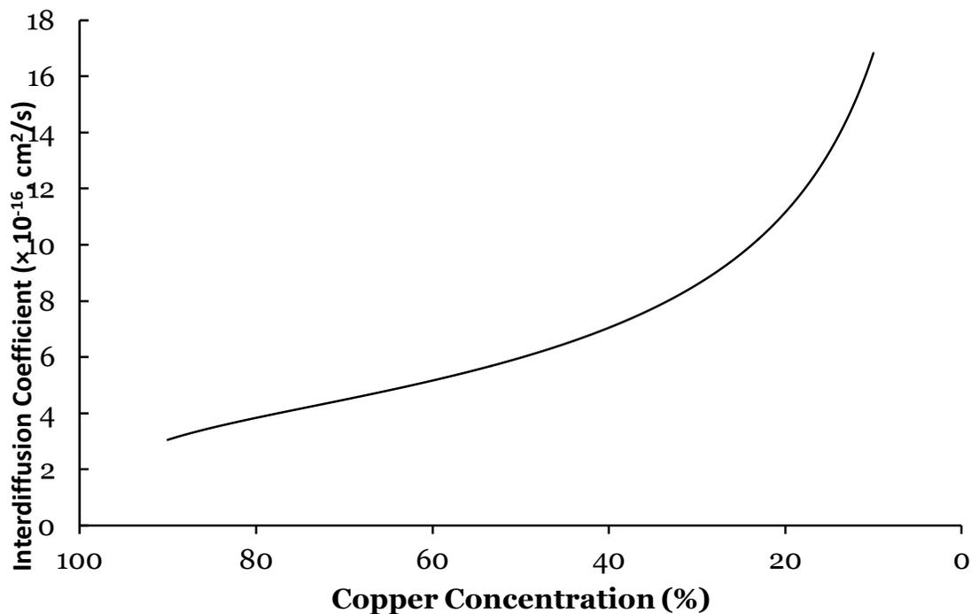
**Figure 6(b):** Interdiffusion coefficient as a function of atomic concentration of copper in the 200°C annealed sample calculated using equation (3).
