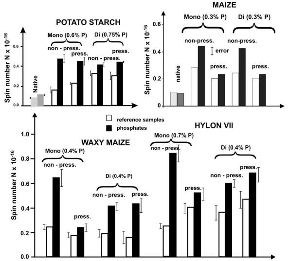
Fig. 9. Effect of multi-step modification (phosphorylation followed by high pressure treatment and heating at 210°C) on the number of radicals generated in starches of various botanic origin (potato [25] and normal maize [5]) and of various content of amylose [26] (normal maize, waxy maize and HylonVII).
