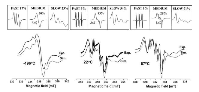
Fig. 4. Temperature dependence of the EPR spectrum of PBN adduct with short-lived radicals generated in native maize starch at 180° C [5].
