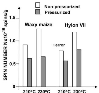
Fig. 7. Influence of high pressure treatment on the number of radicals generated at  $210^{\circ}$  C and  $230^{\circ}$  C in waxy maize and Hylon VII.
