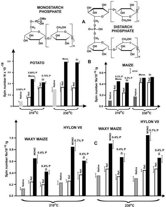
Fig. 5. Effect of phosphorylation on the number of relatively stable radicals generated thermally in starches of various botanic origin and various amylose content [5, 25, 26].
