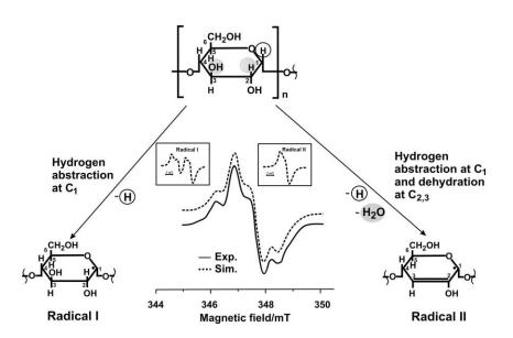
Fig. 2. Mechanism of the thermal generation of relatively stable radicals in starch.
