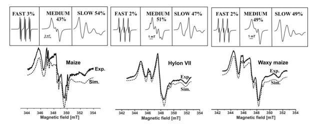
Fig. 3. EPR spectra of the PBN adducts of short-lived radicals generated at 180° C in native maize, Hylon VII and waxy maize. Upper inserts represent particular components [5, 6].
